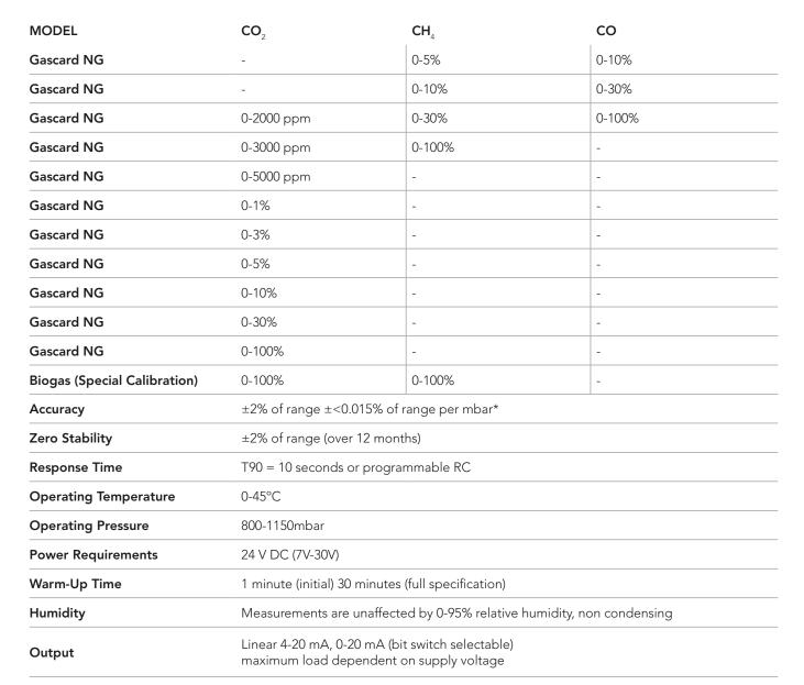
The Gascard NG can also be supplied with an Ethernet option and additional accessories which include a digital display kit and a 24 V pump.
