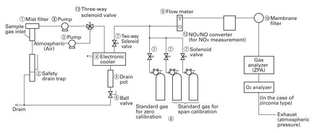
\*1) For NO, SO<sub>2</sub>, or 0–200 ppm range CO measurement, be sure to use an electronic cooler to keep the moisture content below the level saturated at 2°C.
